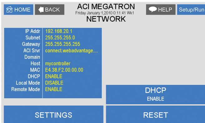
**SETTINGS** - This menu is used for setting up the remote WebAdvantage communications and is covered in a separate manual.
