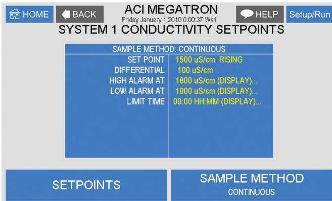
**SET POINT** - What reading turns the relay on.
