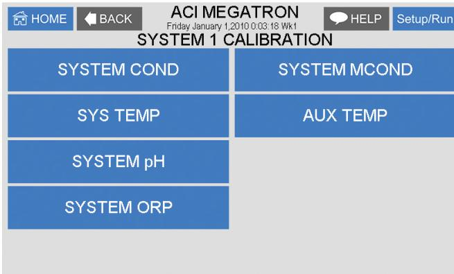
**CALIBRATION** - For adjusting the actual reading values of the available analog probe inputs, such as conductivity, pH, ORP or temperature.
