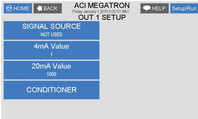
**SIGNAL SOURCE** - Select which probe reading the mA will use as its reading source.
