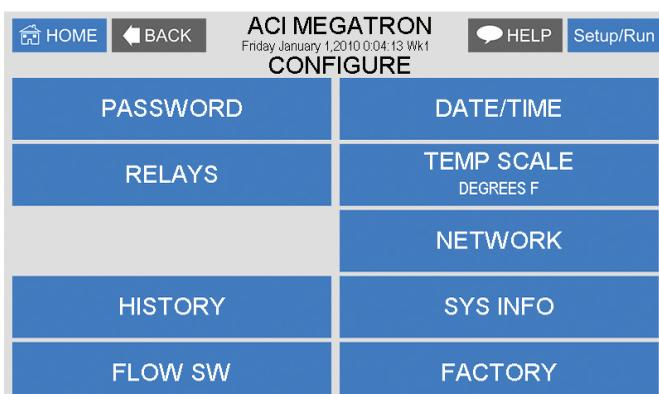
Provides access to menus to set-up passwords, relay activation, temp scale, display contrast, flow switch, inputs, history time stamps, factory set-up and system information.
