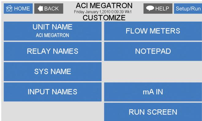
**RUN SCREEN** - Allows the user to select what will be shown on the screen while the controller is in the RUN mode, such as displaying temperature readings, water meter totals for a particular system, or the conductivity units of measure.
