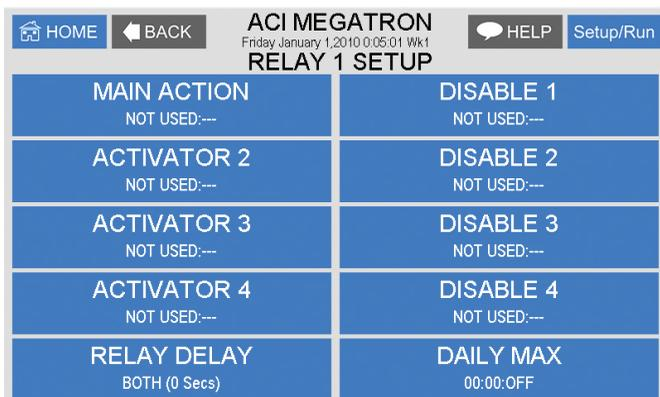
**CONFIGURE RELAYS** - This menu lets you choose a **Main Action** or function (timer 1, conductivity, alarms etc...) to activate a relay.
