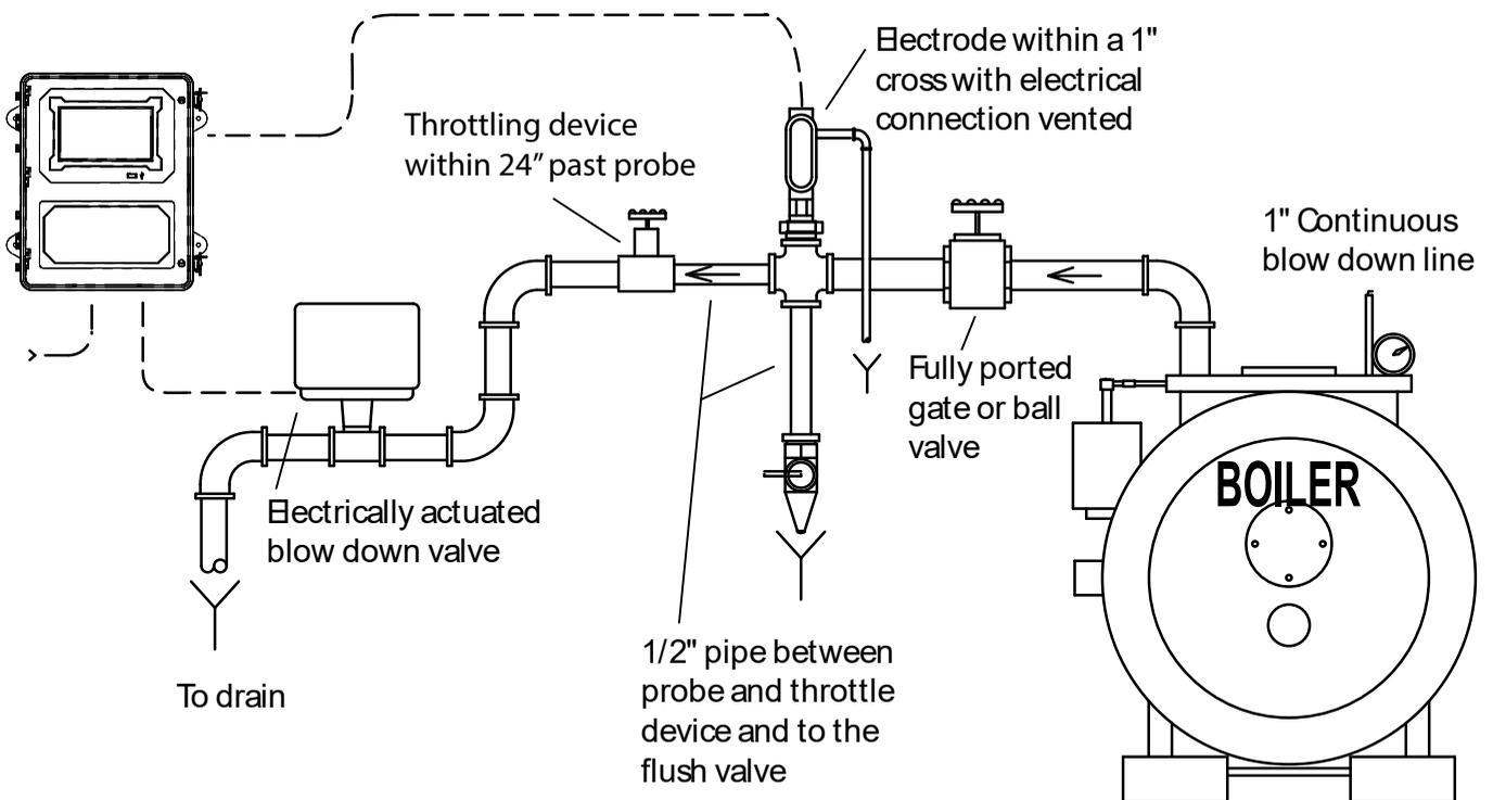
**Warning - Do not use on bottom blowdown lines, only continuous or surface blowdown lines.**
