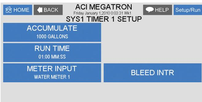
**ACCUMULATE** - The number of gallons or liters from water meter to count before activating timer.
