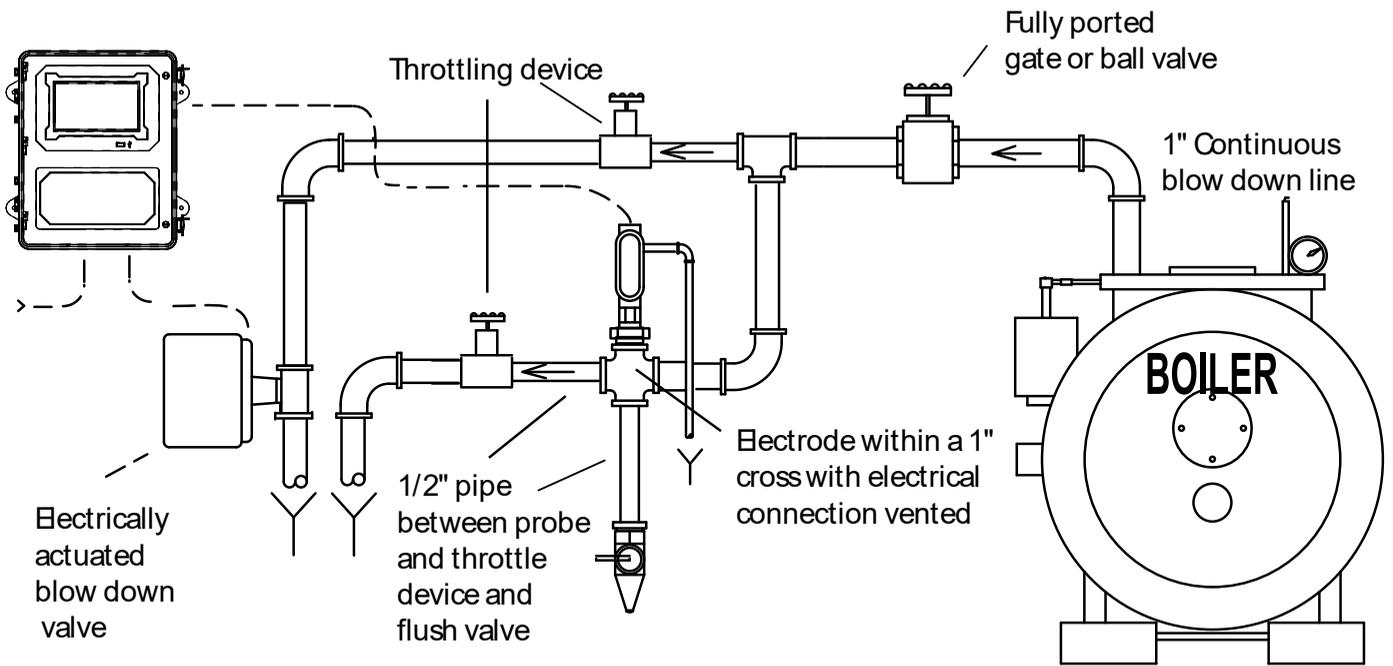
**Warning - Do not use on bottom blowdown lines, only continuous or surface blowdown lines.**
