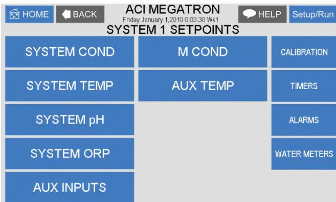
**SET POINTS** - For setting the relay set points for the available analog probe readings such as conductivity, pH, ORP, or temperature.
