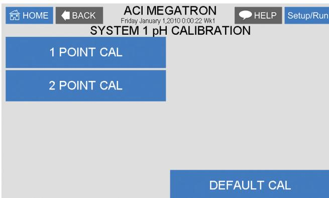
**1 POINT** - With a clean probe on-line seeing the system's water enter the known (tested from a calibrated handheld tester) value.
