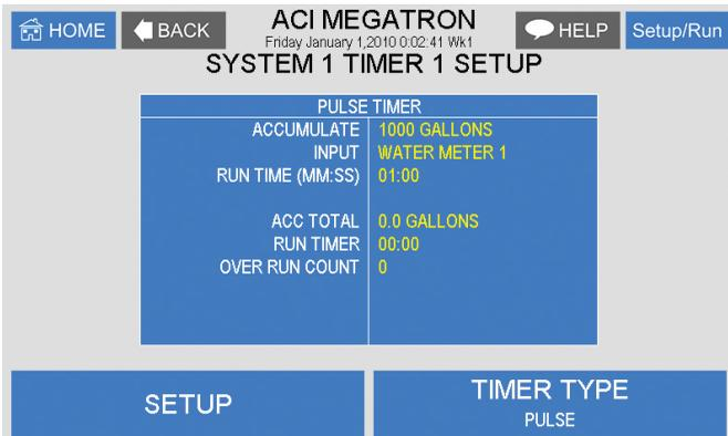
Each timer type selected will have its own unique Set Up submenu with additional selections specific to the type of timer selected. The page displayed before entering the Set Up menu of a timer provides an overall review of the timers current settings.
