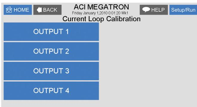
4-20mA outputs can be calibrated to ensure that the output generated by the controller and received by the external device match. With a voltmeter connected across the out and return wires (see page 7) of the 4-20mA output channel, to be calibrated, go into the output's Low or High calibration.
