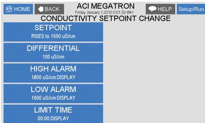
Tower systems with this option have an additional menu on the review page labeled SAMPLE METHOD. The sample method pop-up screen allows the user to select continuous or cycles control. With cycles selected under Settings, a best and worst cycles value is attached to a best and worst make-up conductivity value. The controller will control the cycles proportionally between the two cycles values as the make-up conductivity changes between the two identified values.
