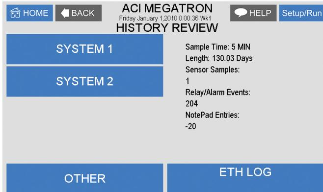
**NOTE:** The history can be reset by going to the configure menu and entering a different sample interval. After the new sample interval has been set, the onboard history is reset.
