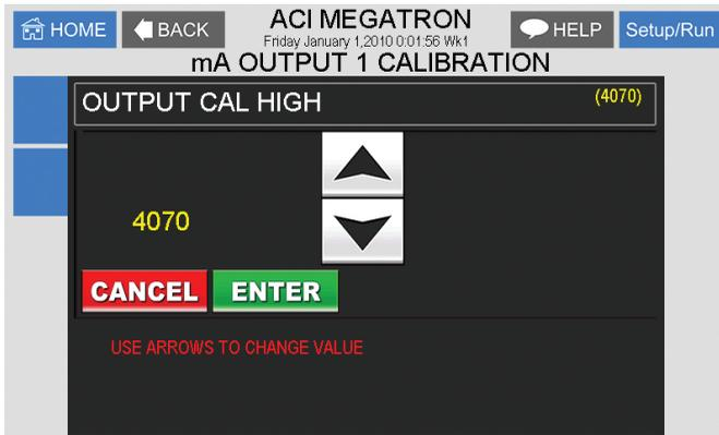
While in the High or Low calibration pop-up screen use the up and down arrows to change the output value being read with the voltmeter. Adjust the High value for the 20-mA reading and the Low value for the 4-mA value.
