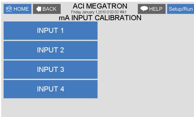
4-20mA inputs can be calibrated to ensure that the input seen by the controller from the external device match. It also allows for setting the 4-20mA input into a number range that relates to the value being read.
