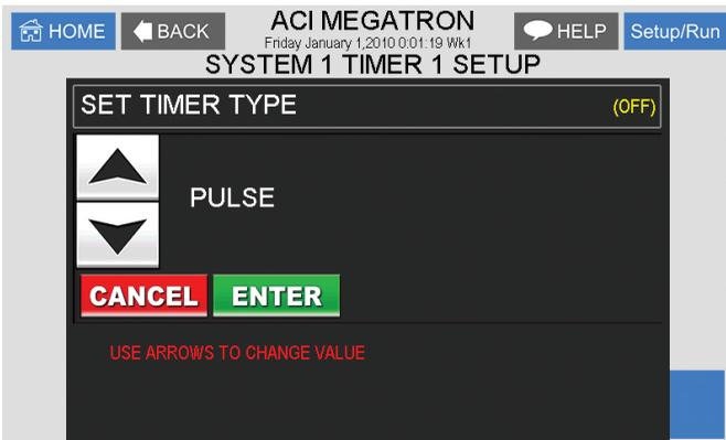
**Pulse** - A water meter activated timer.
