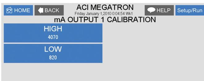
The number displayed in the Calibration dialog box can range from 0-4,095, with 800 equal to 0 mA output, and 4,030 equal to 20 mA. This number range of 0-4,095 is the raw digital-to-analog (D/A) values and is strictly used for reference. The D/A numbers that you get will vary based on your installation conditions.
