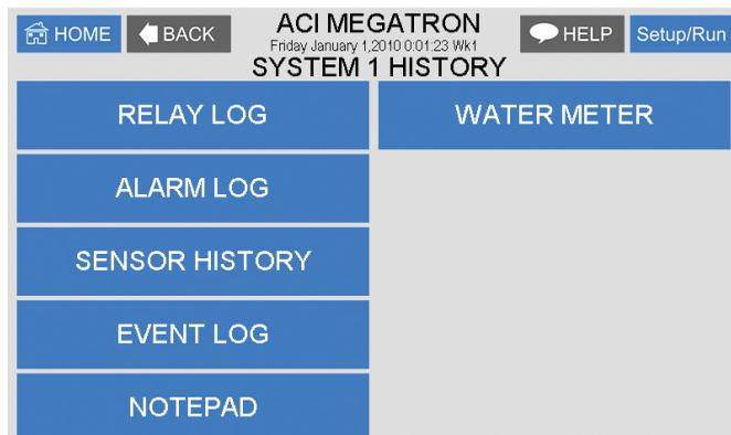
**RELAY LOGS** - Relay activations displayed in a log form. Arrow up to advance through the log.
