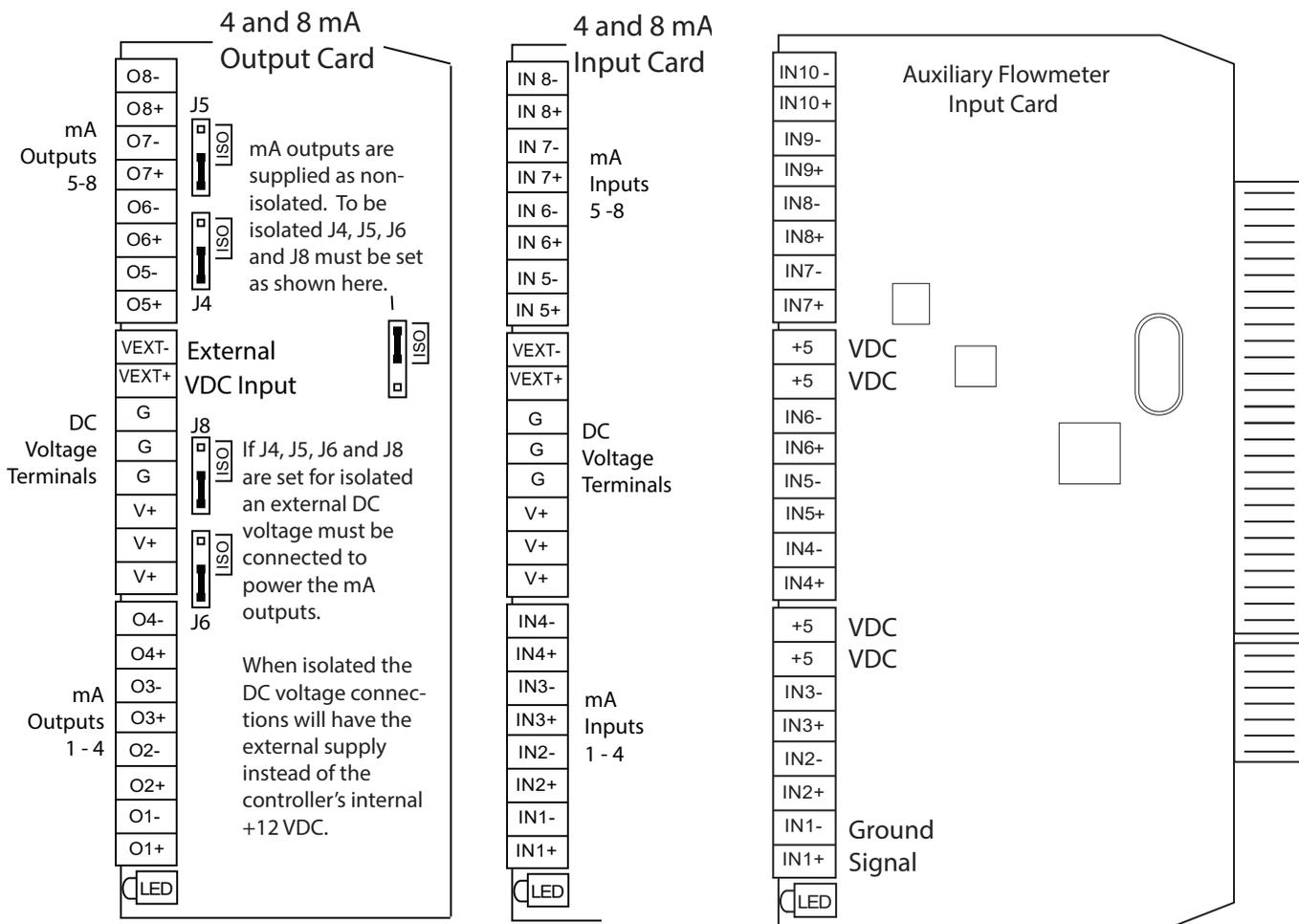
**NOTE:** Older green versions of the 4 input cards supply +12 VDC and ground on the voltage terminals, and newer blue versions supply +12 and -12 VDC instead of ground on the "G" positions, if not configured for isolated voltage.
