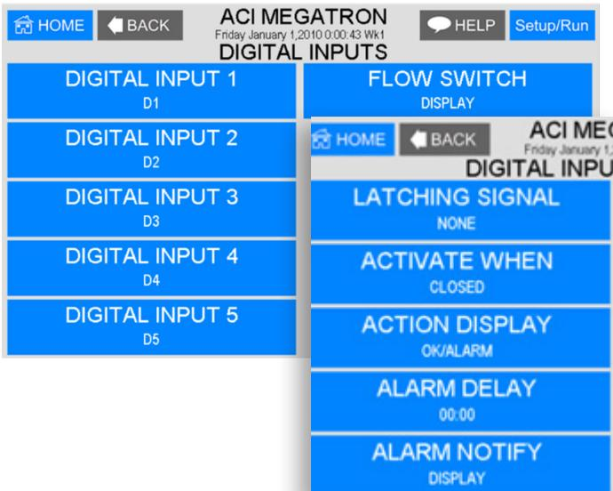
**LATCHING SIGNAL** - Allows a digital input to stay Active until a second latched input becomes active.
