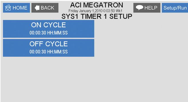
**ON CYCLE** - The amount of the defined time that the timer is to be on.
