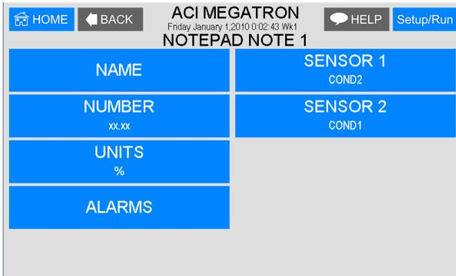
**SENSOR 1** - The first sensor reading or Notepad value to be used in the calculation.
