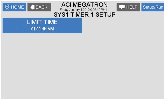
**LIMIT TIMER** - This timer starts when the conductivity bleed starts and turns off when the bleed stops or until the limit time has been reached. The time can be set in MM:SS.
