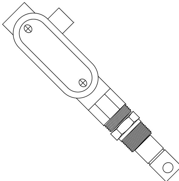
**Wiring Note:** BE-4RTD probes require a 6-conductor cable from controller to probe; BE-32 probes only require a 2 conductor cable.
