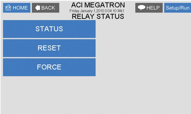
**STATUS** - Allows for viewing accumulated relay ON times, temporary forcing relays ON or OFF or seeing which relay is on.
