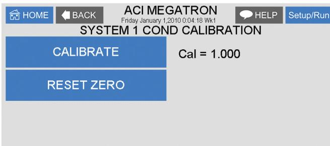
**CALIBRATE** - With a clean probe on-line seeing the system's water enter the known (tested from a calibrated handheld tester) value.
